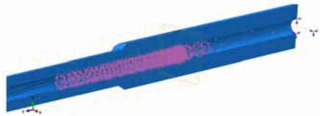
Figure 8. Applied loads on the interior surfaces
