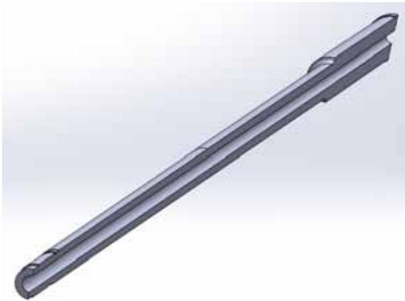
Figure 5. CAD models of the barrel without grooves
