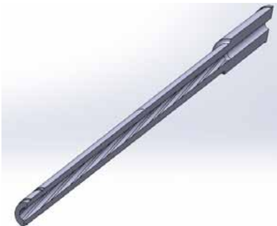
Figure 6. CAD models of the barrel with grooves
