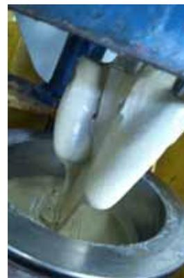
Figure 3. Uncured propellant with a proper pot life
