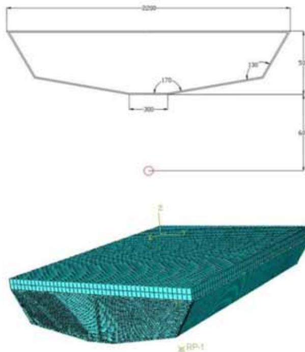
**Figure 2.** V-hull geometry and finite element mesh for the numerical model and the FEM vehicle model and the position of the explosive charge when  $\alpha=170^\circ$  and  $\beta=130^\circ$
