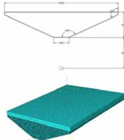
Figure 5. V hull geometry and finite element mesh for the numerical model and the FEM vehicle model and the position of the explosive charge when  $\alpha=155^\circ$  and  $\beta=120^\circ$
