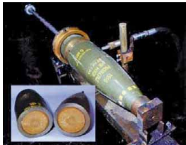
Figure 9. AWJ application for 155 mm projectiles [43]
