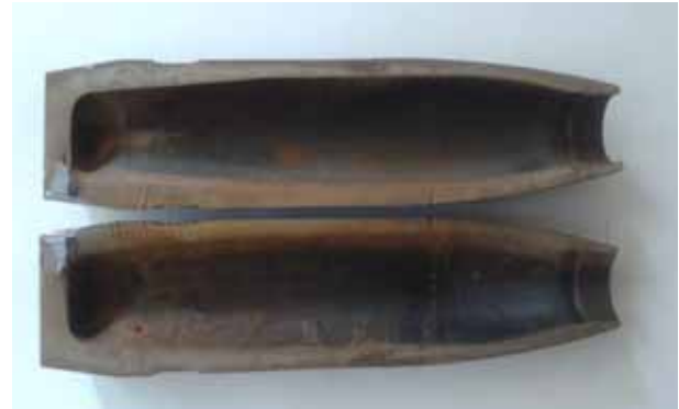
Figure 7. Projectile case after cutting with AWJ
