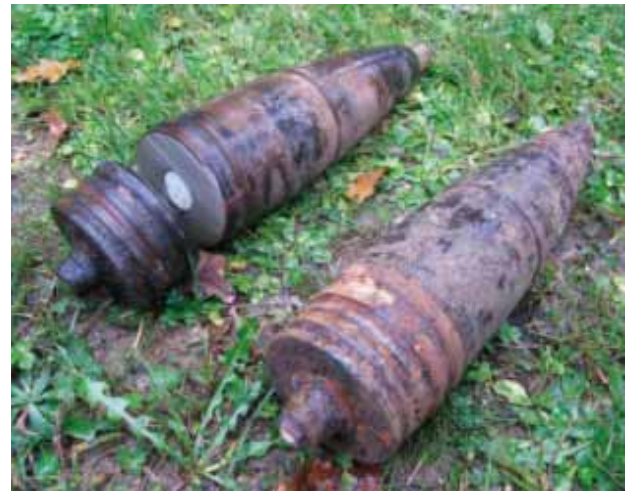
Figure 11. Implementation of AWJ cutting in the disassembly process of the UXO [47]
