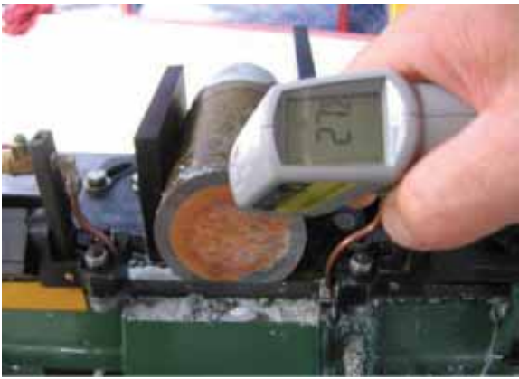
Figure 13. Monitoring of temperature during the sawing of the projectile and explosive charge [38]
