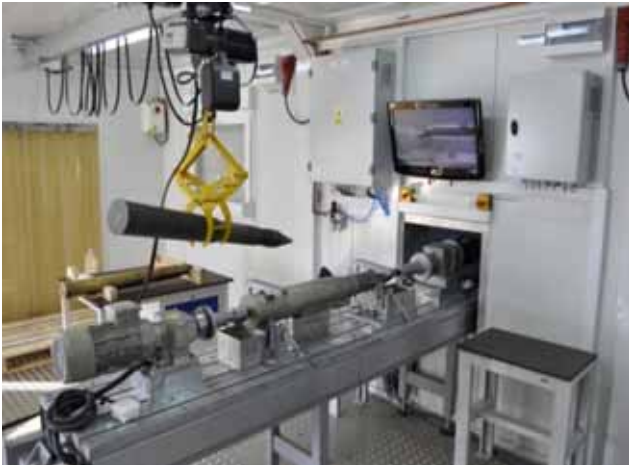
Figure 3. Illustration of an automated process for disassembling EO into subassemblies and elements [24]
