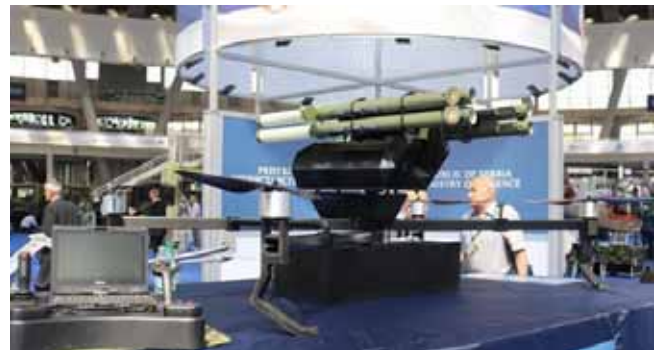
Figure 11. New armed quadcopter with M80 anti-tank unguided rockets
