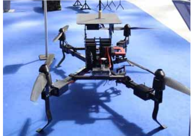
Figure 7. Drone-carried jammer for jamming tactical communications
