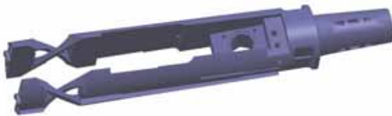
Figure 4. Elastic element with a pair of symmetrical cross-flexures
