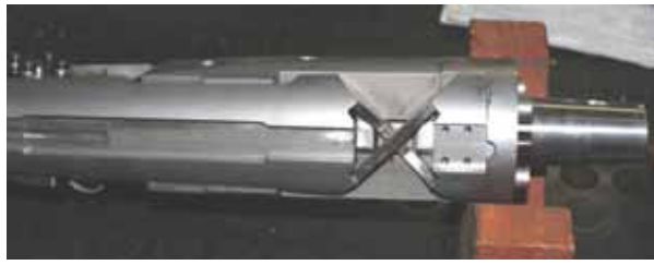
Figure 13. Elastic element with variable cross-section strips
