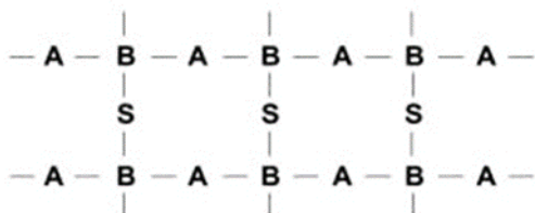
Figure 5. Chemically cross-linked molecular chains of polyester resin
