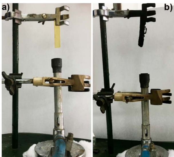
Figure 7. a) Neat UPe resin before UL 94V test and b) UPe/KLP(c) composite after UP 94V test
