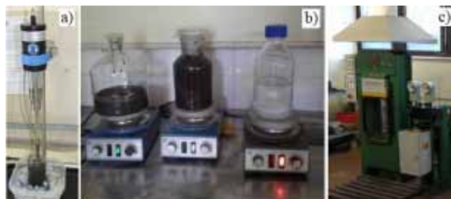
Figure 3. a) Ultrasonic dispersion of WS 2 nanoparticles, b) dissolving PVB in ethanol with and without nanostructures of WS 2 , c) Beliše Thermal Press
