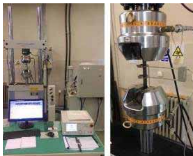
Figure 5. Tensile testing on Shimadzu Servo Pulser
