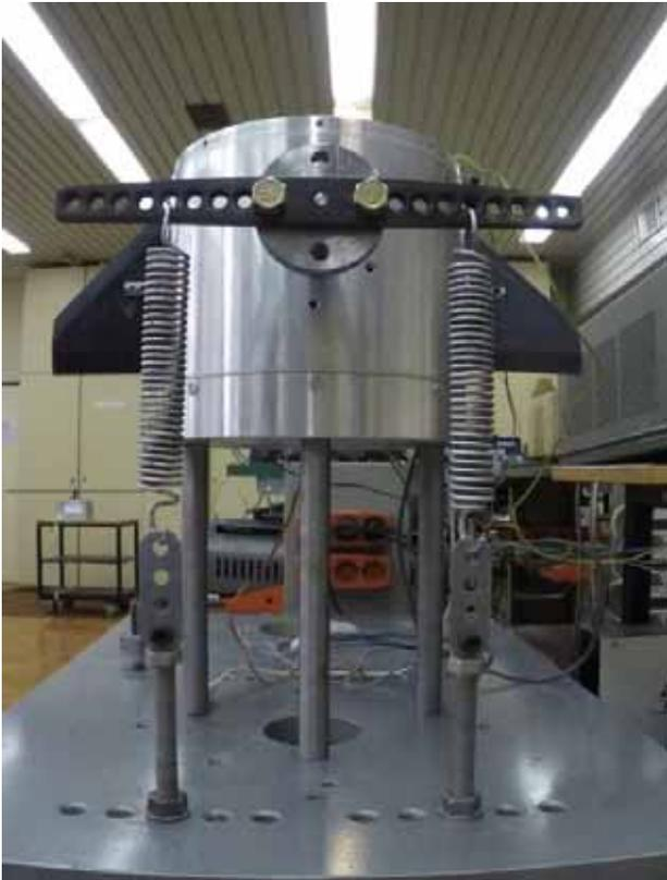
Figure 2. The missile flight control module, on the test bench
