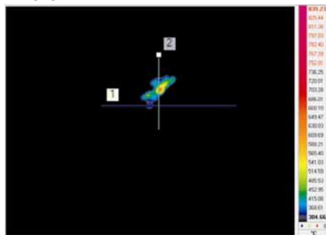
Figure 5. Thermal image of igniting coal captured by FLIR SC7200 camera, sequence Capture1455
