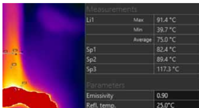
Figure 12. Thermal image captured by FLIR CAT S60 camera after combustion: Left – burning paper (cellulose); right – maximum temperature along flame marker line was determined
