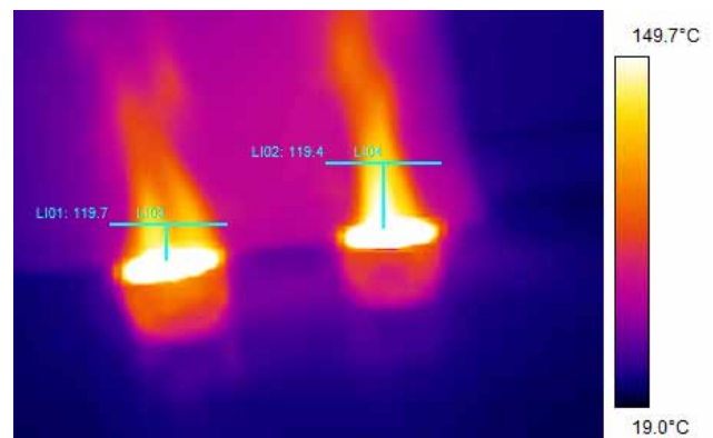
Figure 1. Thermal image of two burning liquids captured by FLIR CAT S60 camera: Left – pure plum brandy; right – mixture of plum brandy and alcohol
