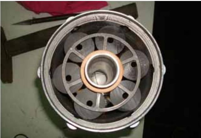
Figure 14. Propellant tubes around the central tube
