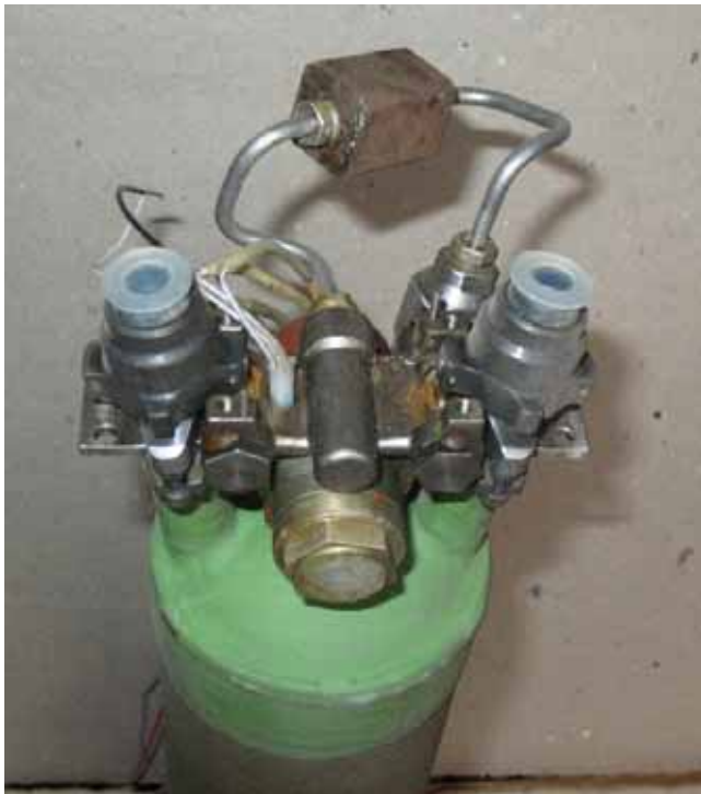
Figure 3. TVC system with a small chamber for measuring the pressure [8]
