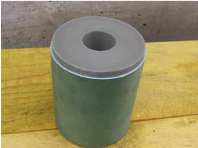
Figure 17. Propellant grain for the rocket motor Bumar
