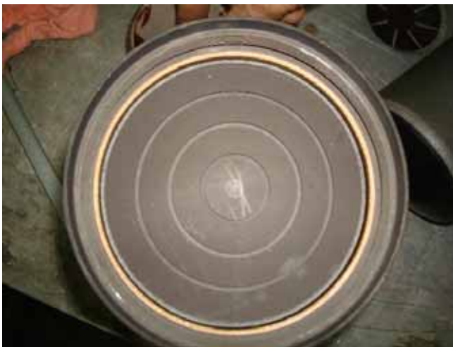
Figure 18. Propellant grain for the additional sustainer
