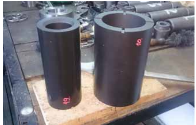
Figure 23. "Telescopic" propellant grains
