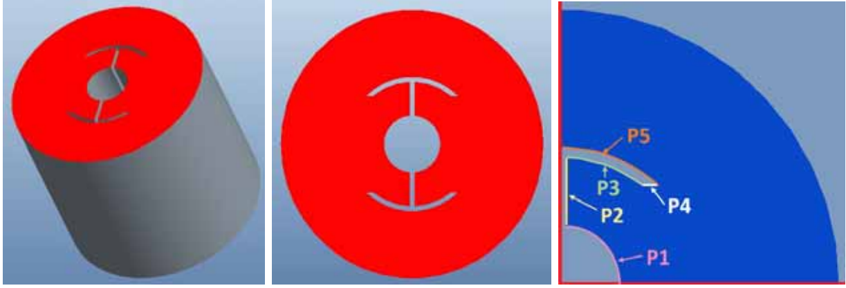
Figure 3. Appearance of the propellant grain at the start of the first phase of combustion with the dimensions on which the mathematical model of combustion is concerned
