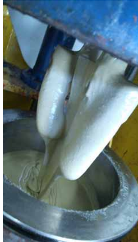
Figure 7. Uncured propellant on mixing blades at the end of homogenizing process
