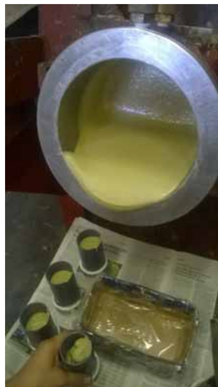
Figure 8. Casting of 2-inch motor case
