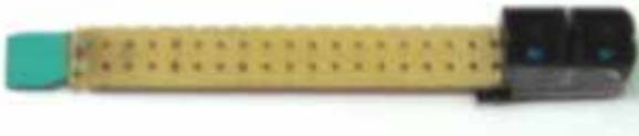
Figure 6. Two CNY70 sensors on a 7 mm wide base board prepared for mounting in a wind tunnel model. The connector is on the left.
