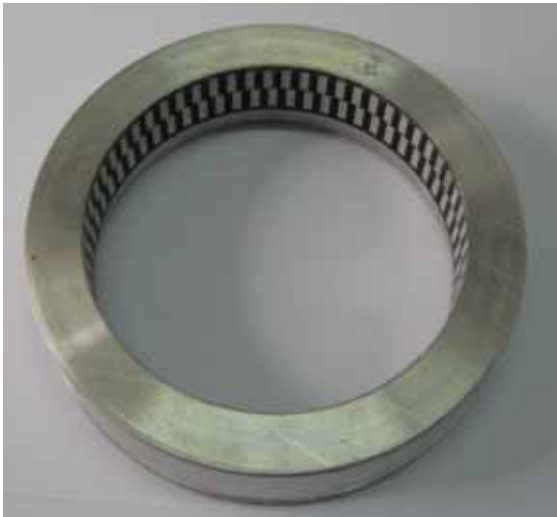
Figure 2. Striped mask attached to a rotating ring used for transducer tests
