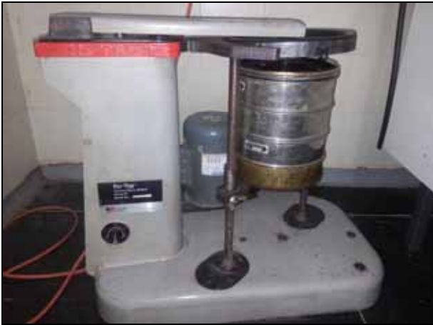
Figure 6. Apparatus for sieving the mixture
