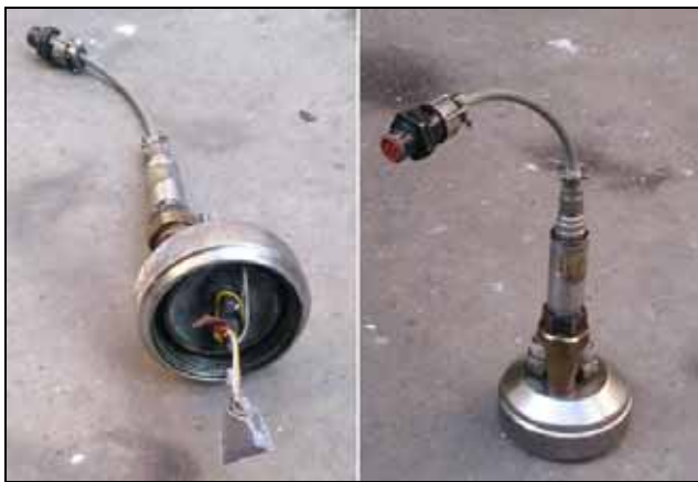
Figure 12. Manometer bomb cover with the igniter and the pressure transducer
