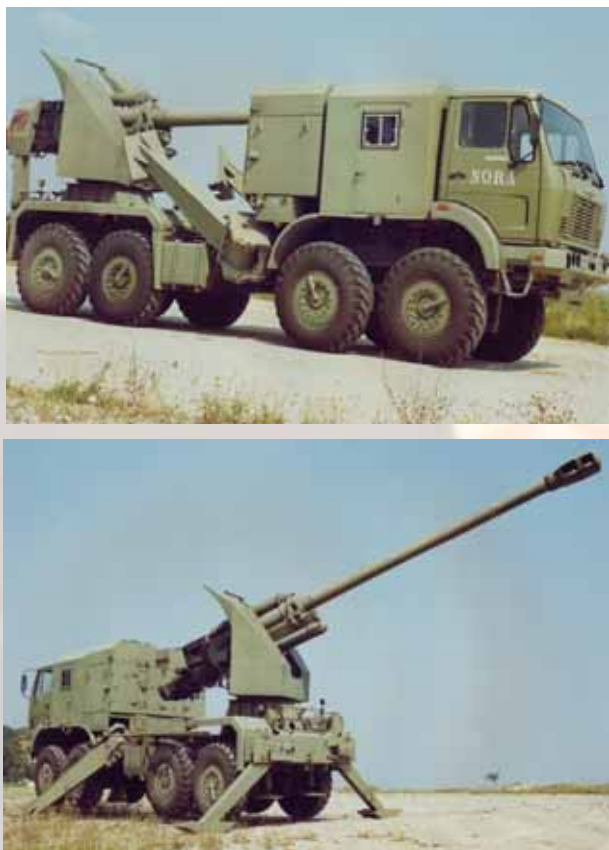
Figure 9. Functional model of the 152 mm NORA-B truck-mounted weapon: travelling configuration (top) and combat position (bottom)
