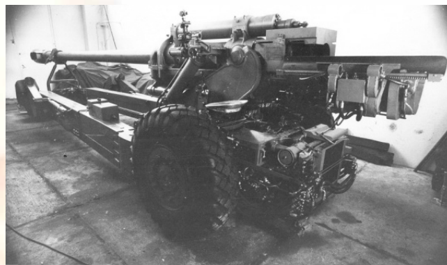
Figure 8. 152 mm NORA-C2 prototype weapon with auxiliary propulsion unit
