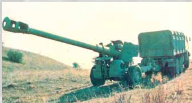
Figure 7. Concept demonstrator of the 152 mm NORA-C1 weapon with auxiliary propulsion unit
