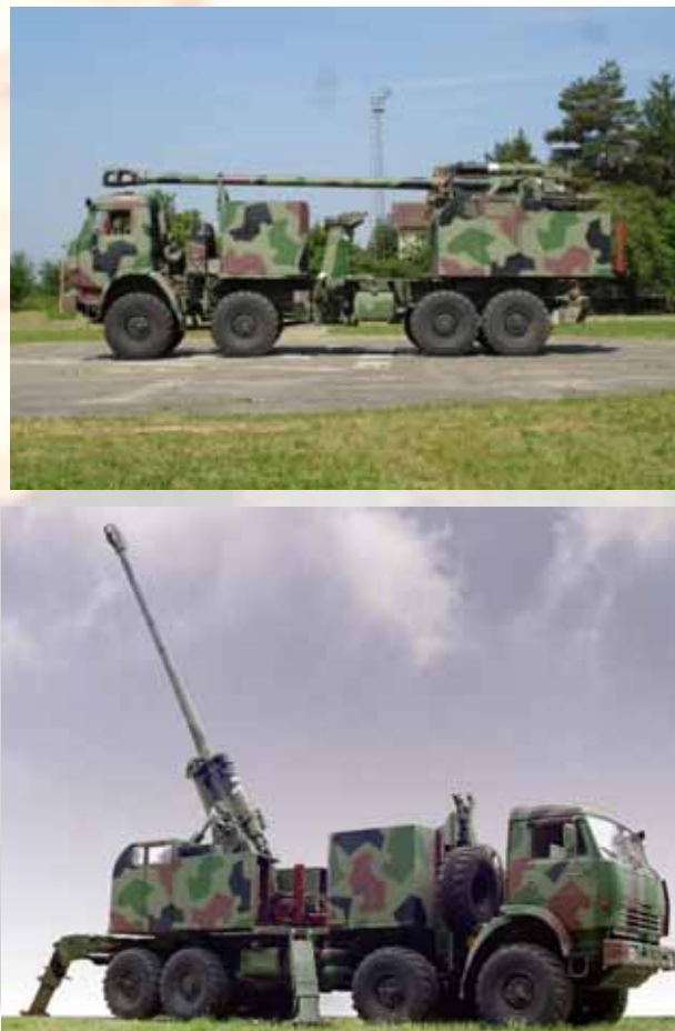
Figure 10. Prototype of the 155 mm NB-52 gun-howitzer: travelling configuration (top), combat configuration (bottom)
