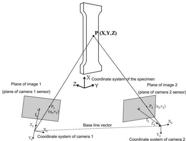
Figure 2. Schematic of the stereometric system.
