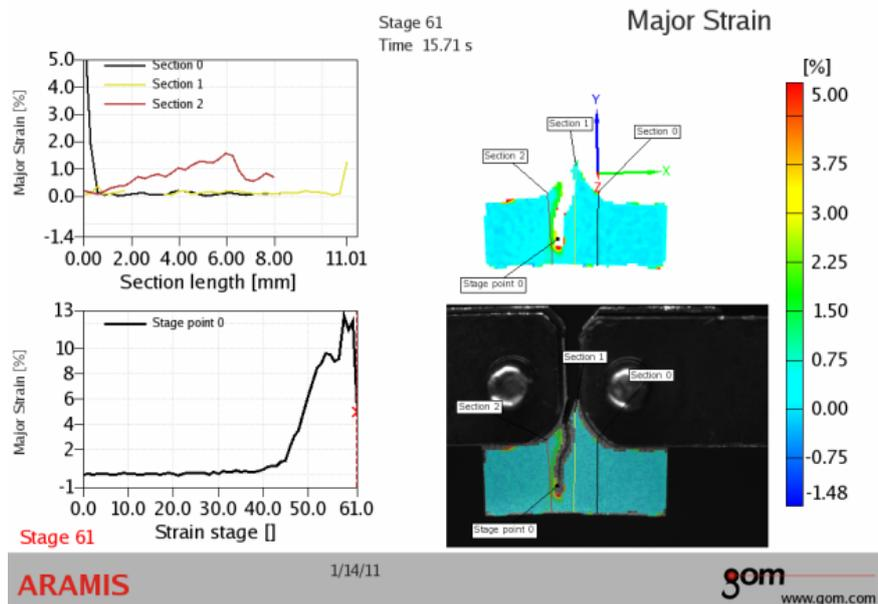
Figure 8. Results for C(T) specimen at the moment of fracture
