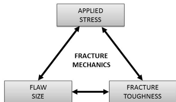
Figure 1. Fracture mechanics triangle [3]
