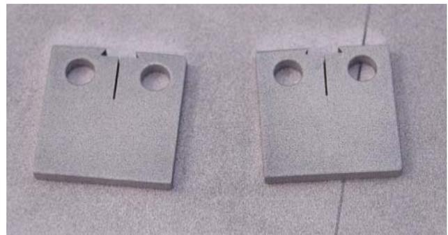
Figure 6. Prepared C(T) specimens
