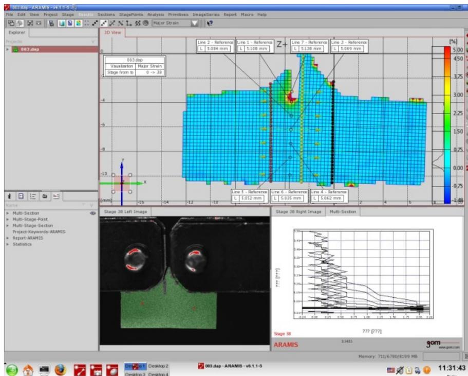
Figure 7. Results for C(T) specimen during crack propagation
