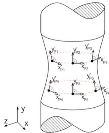
Figure 3. Schematic of the local strain directions
