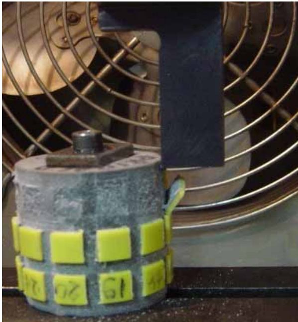
Figure 6. Sample S1 just before the end of testing of the extruded PVC tube-cast HTPB/IPDI propellant bond strength
