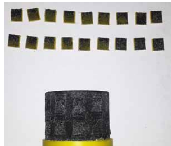
Figure 7. Visual appearance of all single specimen at sample S1 after testing at 20°C
