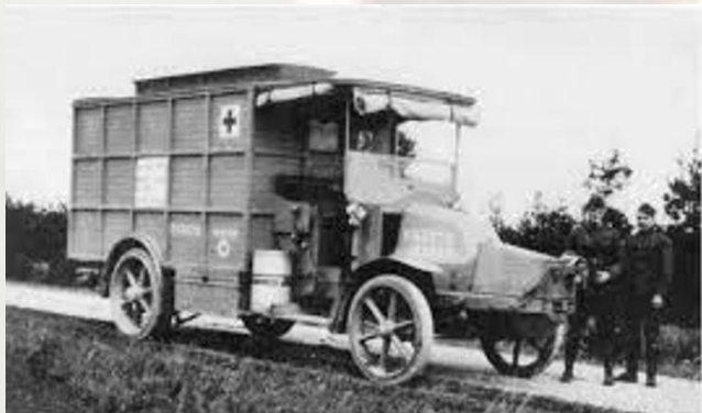
Figure 14. Reno's medical vehicle with roentgen device (Little Curie)
