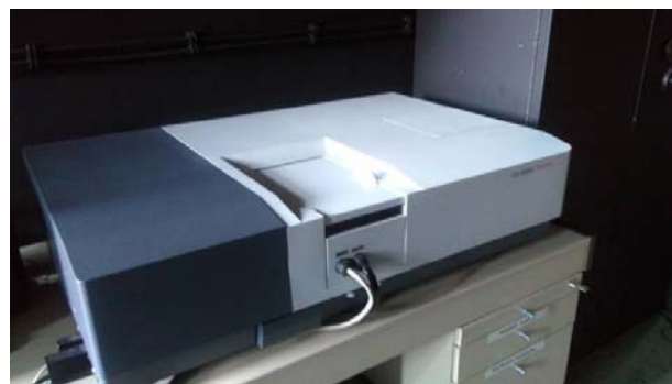
Figure 5. The Shimadzu UV/VIS/NIR spectrophotometer UV 3600
