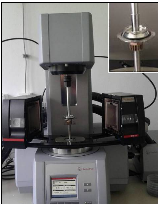
Figure 4. The Modular Compact Rheometer MCR-302
