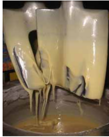
Figure 6. Uncured AP/HMX propellant on the blades
