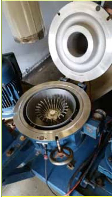
Figure 4. Hammer mill ACM-10 - input housing
