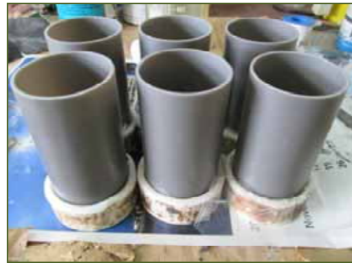
Figure 7. PVC chambers of 2 inch experimental motors (ready for propellant casting)
