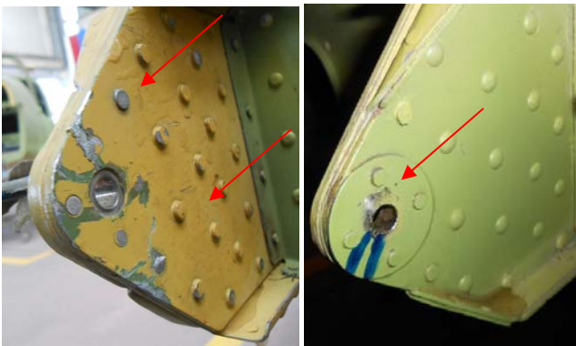
Figure 6. Left – left wing fitting mechanical defects Right – right wing bushing defect of homogeneity
