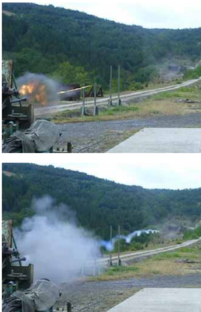
Figure 1. Gas generator units for 37 mm projectile tests
