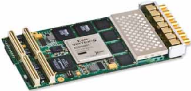
Figure 3. ICS 1554 4-Channel, 160/180 MHz 16-bit ADC PMC Module with Virtex-5 SX95T User Programmable FPGA [5]
