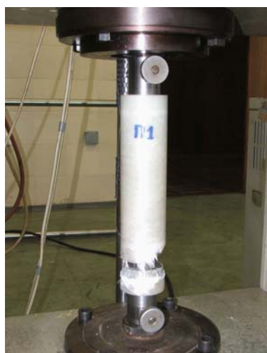
Figure 16. An assembly polyester resin/glass fiber tube ring-cylinder after testing
