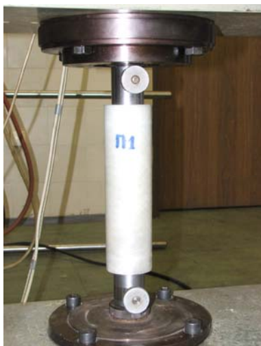
Figure 15. An assembly polyester resin/glass fiber tube-ring-cylinder before testing
