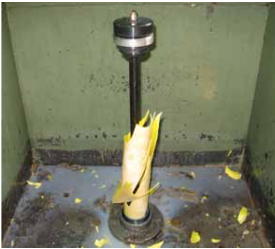
Figure 8. Pipe with the accepted visual appearance after hydraulic burst pressure testing
