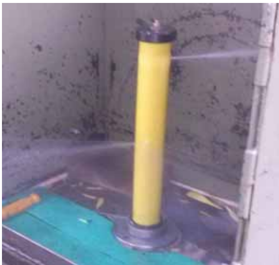
Figure 9. Pipe specimen with the observed impurities during testing under the influence of hydraulic pressure
