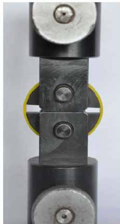
Figure 15. Specific tool for tensile testing with mounted ring shape specimen with the accepted visual appearance
