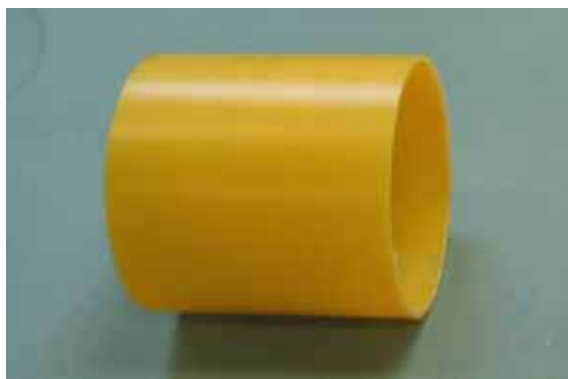
Figure 10. Pipe specimen before testing of the resistance to radial compressive force
