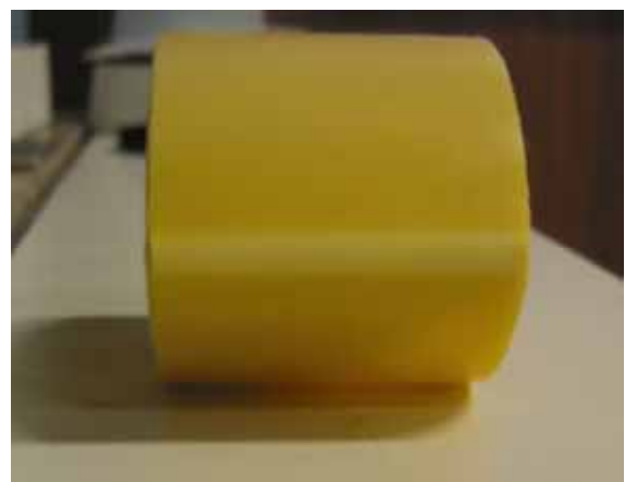
Figure 13. Pipe specimen after testing of the resistance to radial compressive force
