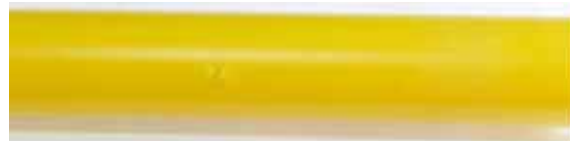
Figure 5. Pipe specimen with the observed impurity
