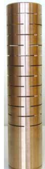
Figure 3. External view of the calibrator for pipe outside diameter 52 mm
