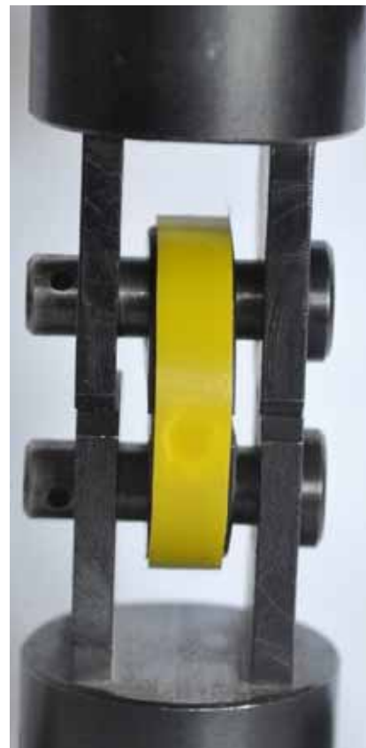
Figure 16. Ring with a round impress, mounted on a specific tool for tensile testing
