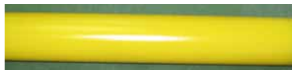
Figure 4. Pipe with the accepted visual appearance
