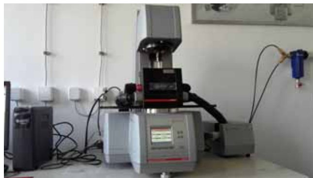
Figure 2. The Modular Compact Rheometer MCR-302 equipped with the temperature chamber
