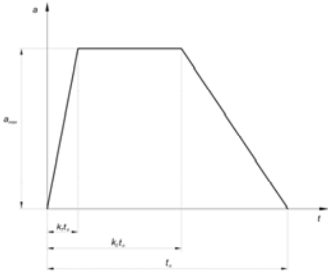
Figure 3. Rocket acceleration vs. time for impulse rocket motor
