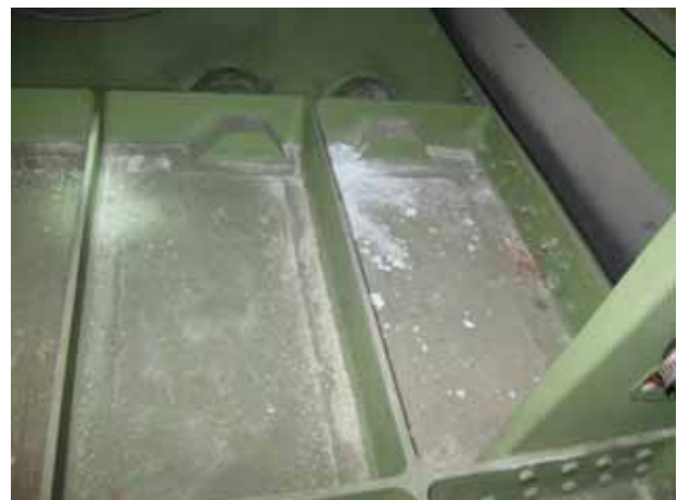
Figure 6. Main fuselage structural assembly attacked by local surface corrosion
