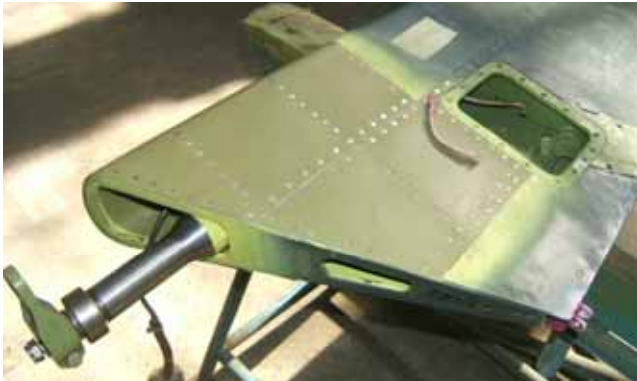
Figure 4. Repaired rudder (after the elimination of severe steel corrosion) ready to be attached to the airplane
