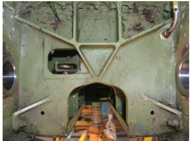
Figure 3. Nose landing gear bay with local points of surface corrosion
