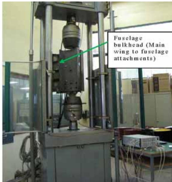
Figure 9. G-4 Fuselage bulkhead during the experimental testing using MTS [6]
