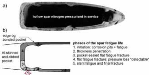
Figure 11. Recovered blade spar fracture surface and phases of the fatigue life [6]
