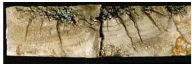
Figure 6. Details of the tail lug fracture, showing intergranular cracking followed by the fatigue. The failure occurred by the fatigue initiating from intergranular cracks on the upper side. The intergranular cracks were heat-tinted. (In October 1990 a Aérospatiale Alouette III helicopter crashed in the Veluwe). [6]
