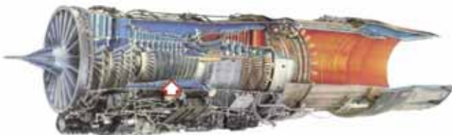
Figure 17. F100-PW-220 engine failure location: RCVV lever arm assembly [6]
