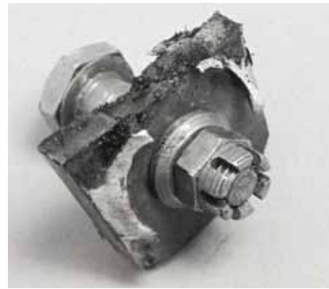
Figure 5. Details of the lug fracture, which was close to welds joining the lug into the airframe. (In October 1990 a Aérospatiale Alouette III helicopter crashed in the Veluwe). [6]
