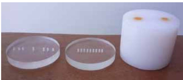
Figure 4. Seven-probes platform (left), nine-probes platform (middle) and the plastic attenuator with two PEP-500 channels (right)
