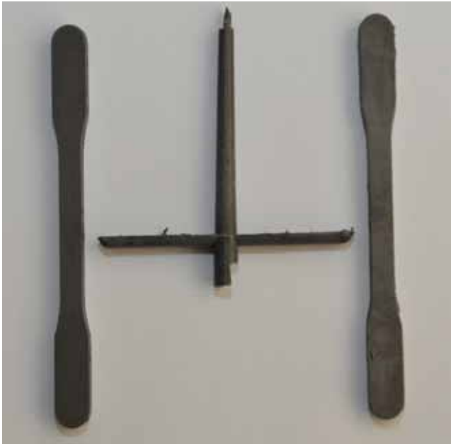
Figure 22. Complete injection moulded specimen
