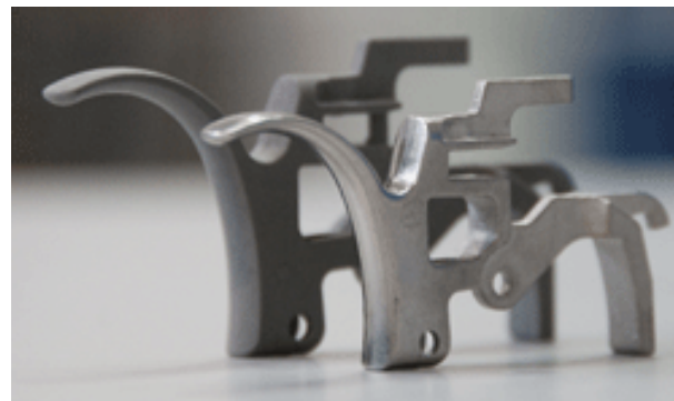
Figure 16. MIM titanium gun trigger (in the background is the "green part" and in the foreground the sintered part)
