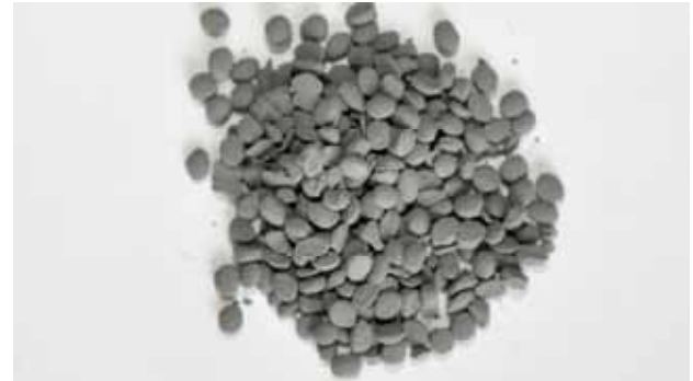
Figure 20. Visual appearance of the Catamold 4605 granule feedstock
