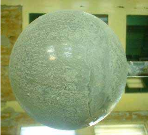
Figure 11. Flow visualization with oil emulsion at M=0.1
