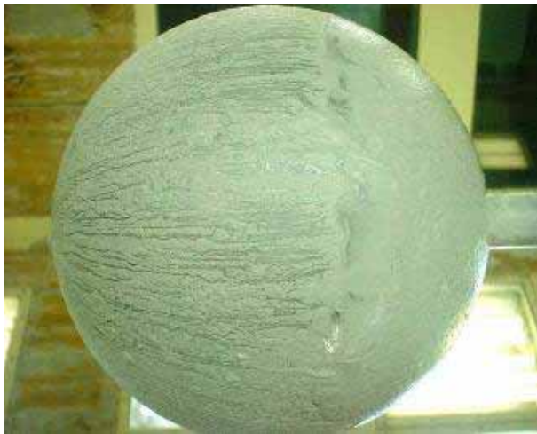
Figure 12. Flow visualization with oil emulsion at M=0.14
