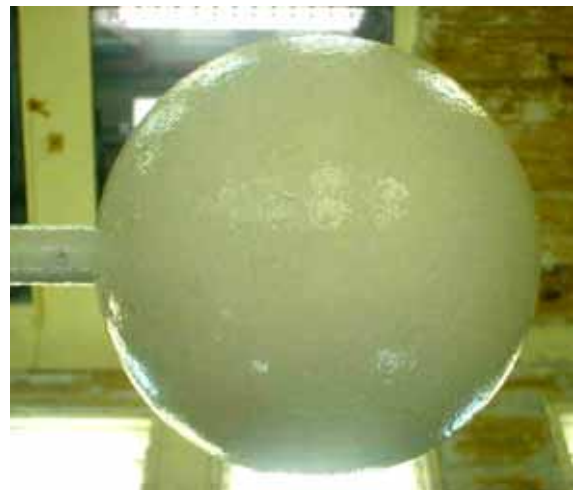
Figure 5. The sphere in the T-35 test section coated with the emulsion Signals from all of the transducers and measuring devices
