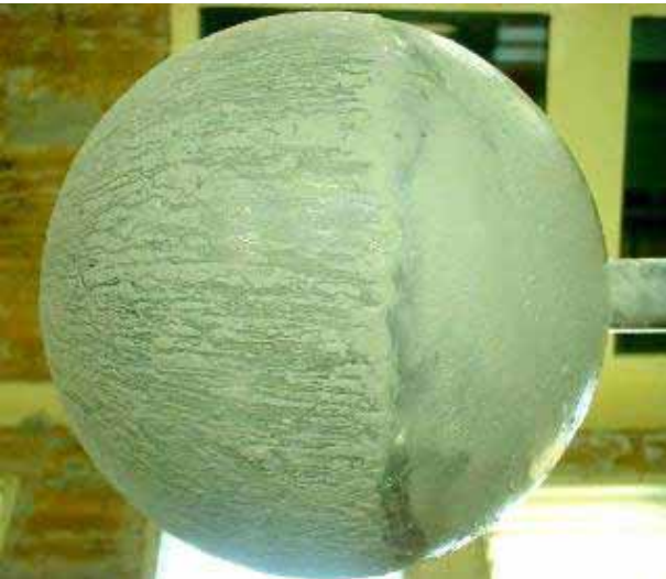
Figure 13. Flow visualization with oil emulsion at M=0.18
