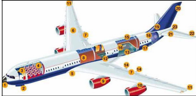
Figure 2. The application of structural sandwich in construction of civil aircraft: 1. Radome 2. Landing Gear Doors and Leg Fairings 3. Galley, Wardrobes, Toilets 4. Partitions 5. Wing to Body Fairing 6. Wing Assembly 7. Flying Control Surfaces 8. Passenger Flooring 9. Engine Nacelles and Thrust Reversers 10. Pylon Fairings 11. Winglets 12. Keel Beam 13. Cargo Flooring 14. Flaptrack Fairings 15. Overhead Storage Bins 16. Ceiling and Side Wall Panels 17. Airstairs 18. Pressure Bulkhead 20. Rudder 21. Horizontal Stabilizer 22. Elevator 23. Tail Cone [3]
