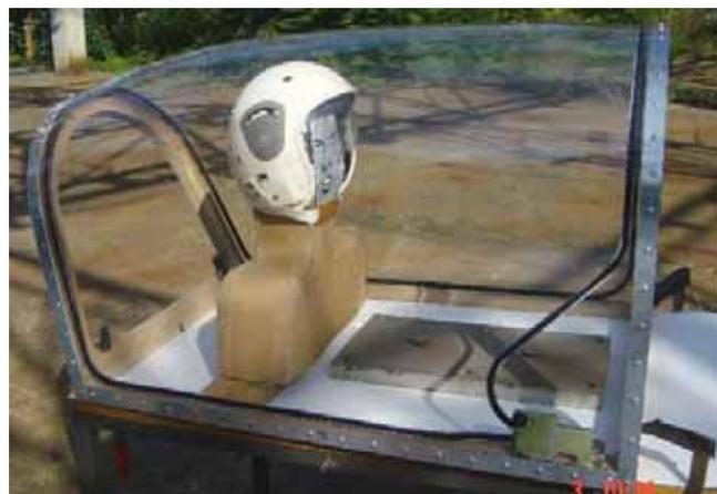
**Figure 17.** Appearance of the canopy before initiating the "Canopy cutting system" detonation of LDSC
