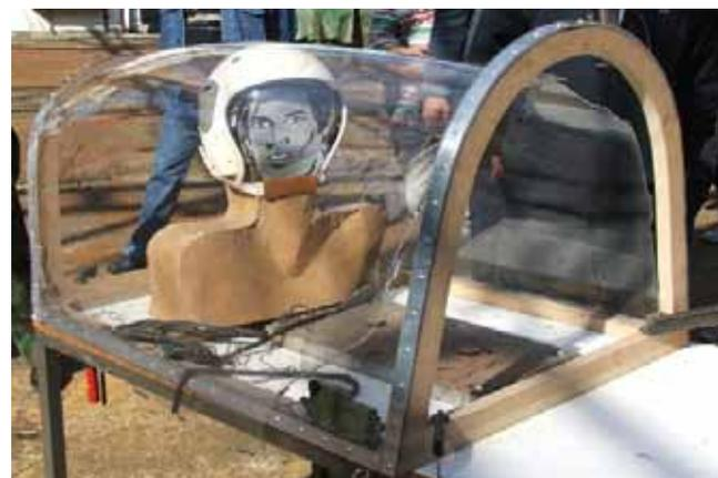
**Figure 18.** Appearance of the canopy after initiating the "Canopy cutting system" (e.g. detonation of LDSC)
