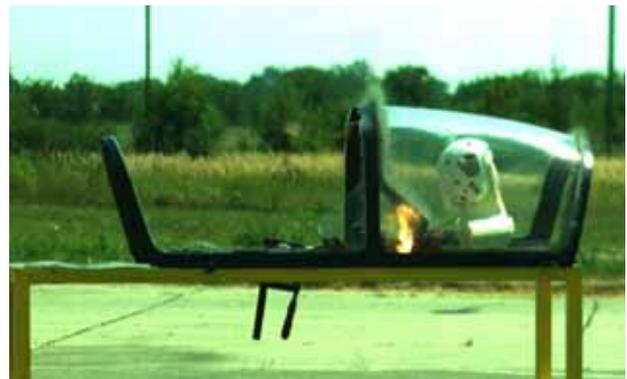
**Figure 23.** Pilot side of the canopy: the initiation of LDSC by initiating cap and cutting the acrylic glass
