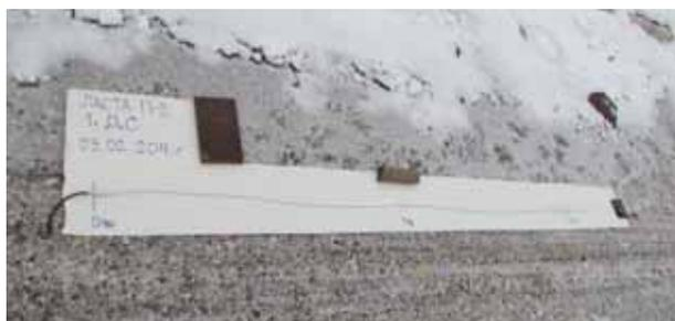
**Figure 15.** Quality tests: LDSC on paper strips before the detonation
