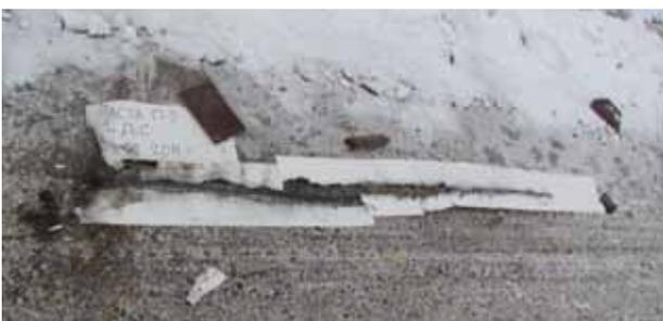
**Figure 16.** Quality tests: Appearance of paper strips after the detonation of the LDSC
