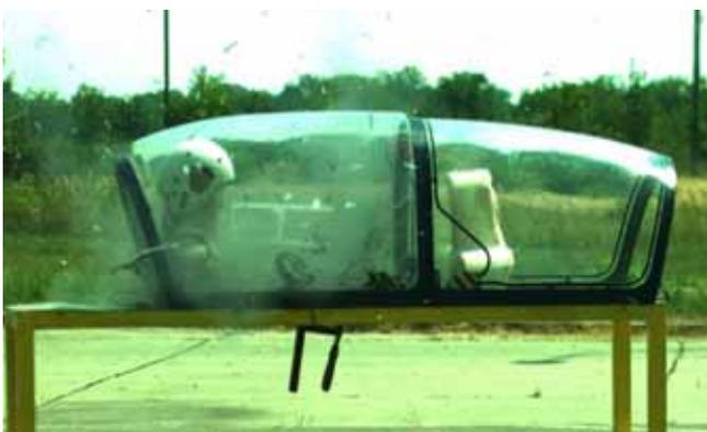
**Figure 21.** Co-pilot side of the canopy: the end of cutting the acrylic glass
