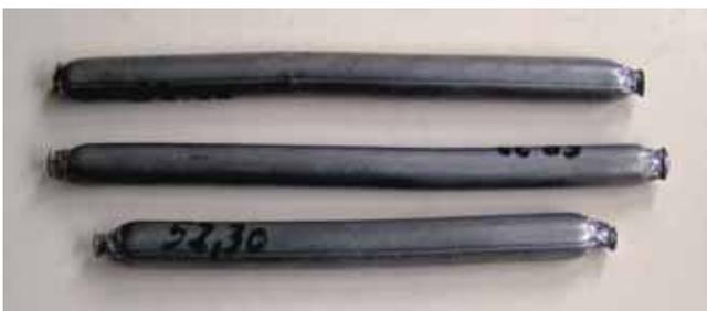
**Figure 2.** The lead tubes filled with graphitized RDX - blanks
