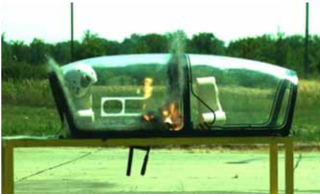
**Figure 20.** Co-pilot side of the canopy: the initiation of LDSC by initiating cap and cutting the acrylic glass of canopy
