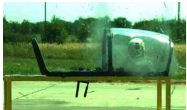
**Figure 24.** Pilot side of the canopy: the end of cutting the acrylic glass
