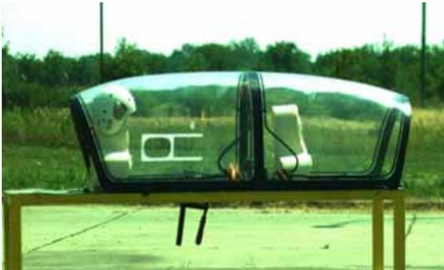
**Figure 19.** Co-pilot side of the canopy: the activation processes of the initiator (initiating cap)
