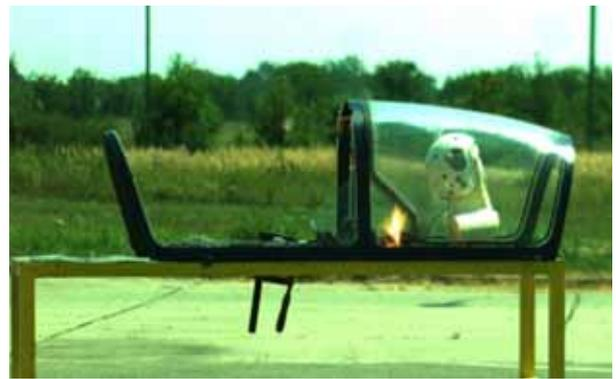
**Figure 22.** Pilot side of the canopy: the activation processes of the initiator (initiating cap)
