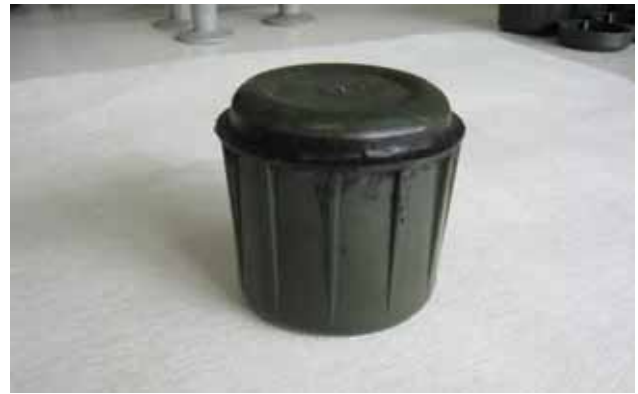
Figure 9. Assembly mark 2/1 (sealed with black silicone)
