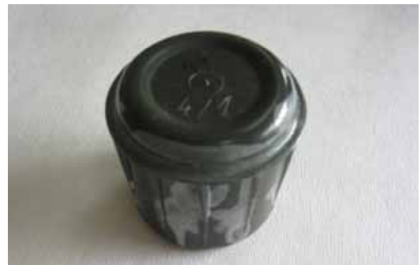
Figure 11. Assembly mark 4/1 (sealed with polystyrene solution)
