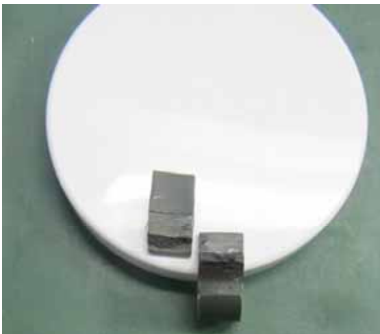
Figure 22. Parts of the specimen cut out from the assembly sealed with the system 2, after tensile testing
