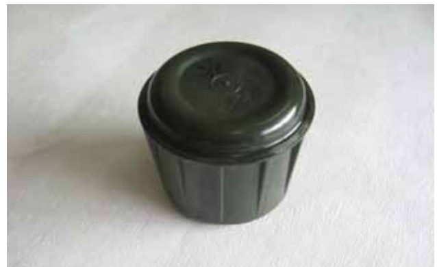
Figure 10. Assembly mark 3/1 (sealed with epoxy resin)
