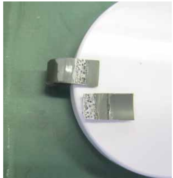
Figure 24. Parts of the specimen cut out from the assembly sealed with the system 4, after tensile testing
