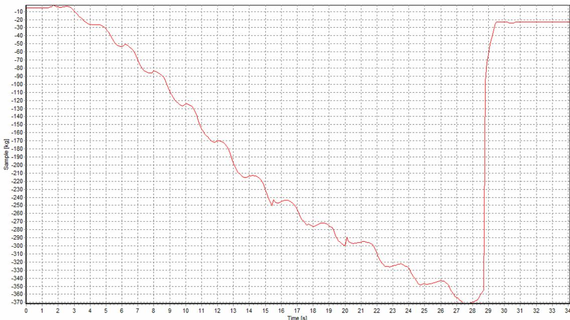
**Diagram 3:**Change of a force value from the start moment of stressing till the moment of breakthrough of cover specimen mark T4/N3
