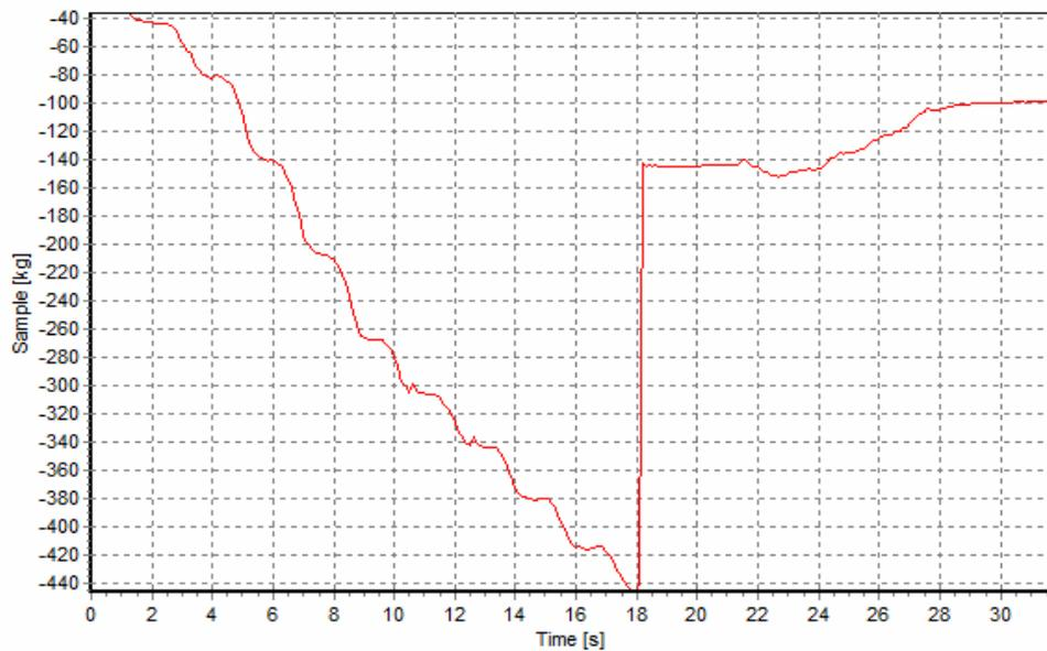
Diagram 1. Change of a force value from the start moment of stressing till the stop of the force action, without breaking cover specimen mark T3/N1
