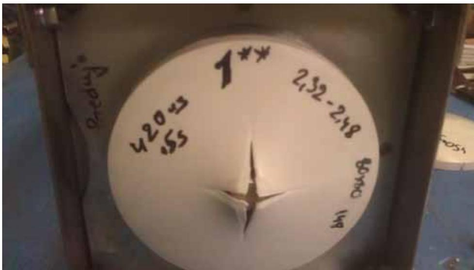
Figure 9. View of cover specimen mark T3/N3 after determining the breakthrough force (420 MPa)
