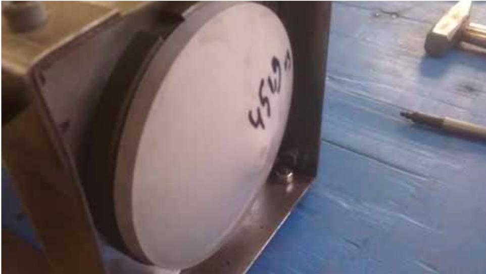
Figure 8. View of cover specimen mark T3/N1 after the action of force of 452 MPa
