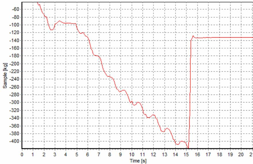
**Diagram 2.** Change of a force value from the start moment of stressing till the moment of breakthrough of cover specimen mark T3/N3
