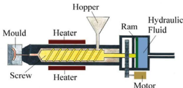
Figure 5. Injection moulding machine
