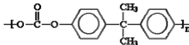
Figure 6. Structure of the polycarbonate basic repeating unit
