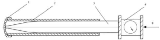
**Figure 7.** Figure of the equipment used for the determination of the breakthrough force of the cover specimens, where : 1-cover specimen, 2-launcher tube, 3-rocket specimen, 4-dynamometer
