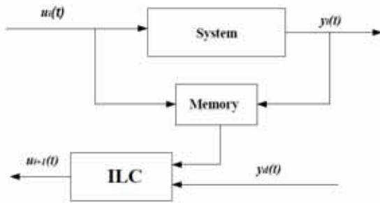
Figure 1. The basic scheme of iterative learning control
