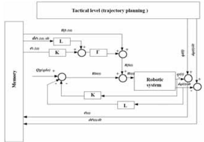
Figure 4. Block diagram of the feedforward-feedback  $PD^\alpha$  type of ILC for a robotic system
