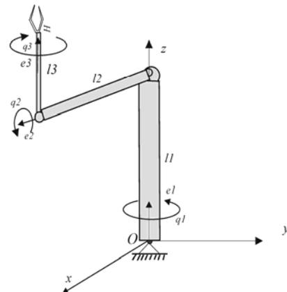
Figure 5. The robotic system with 3 DOF in the reference configuration
