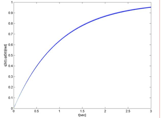
Figure 6. The tracking performance of the system trajectory ( $q(t)$ ,  $k=1,2,3$ : solid line,  $q_d(t)$ ,  $k=1,2,3$ : bold line)
