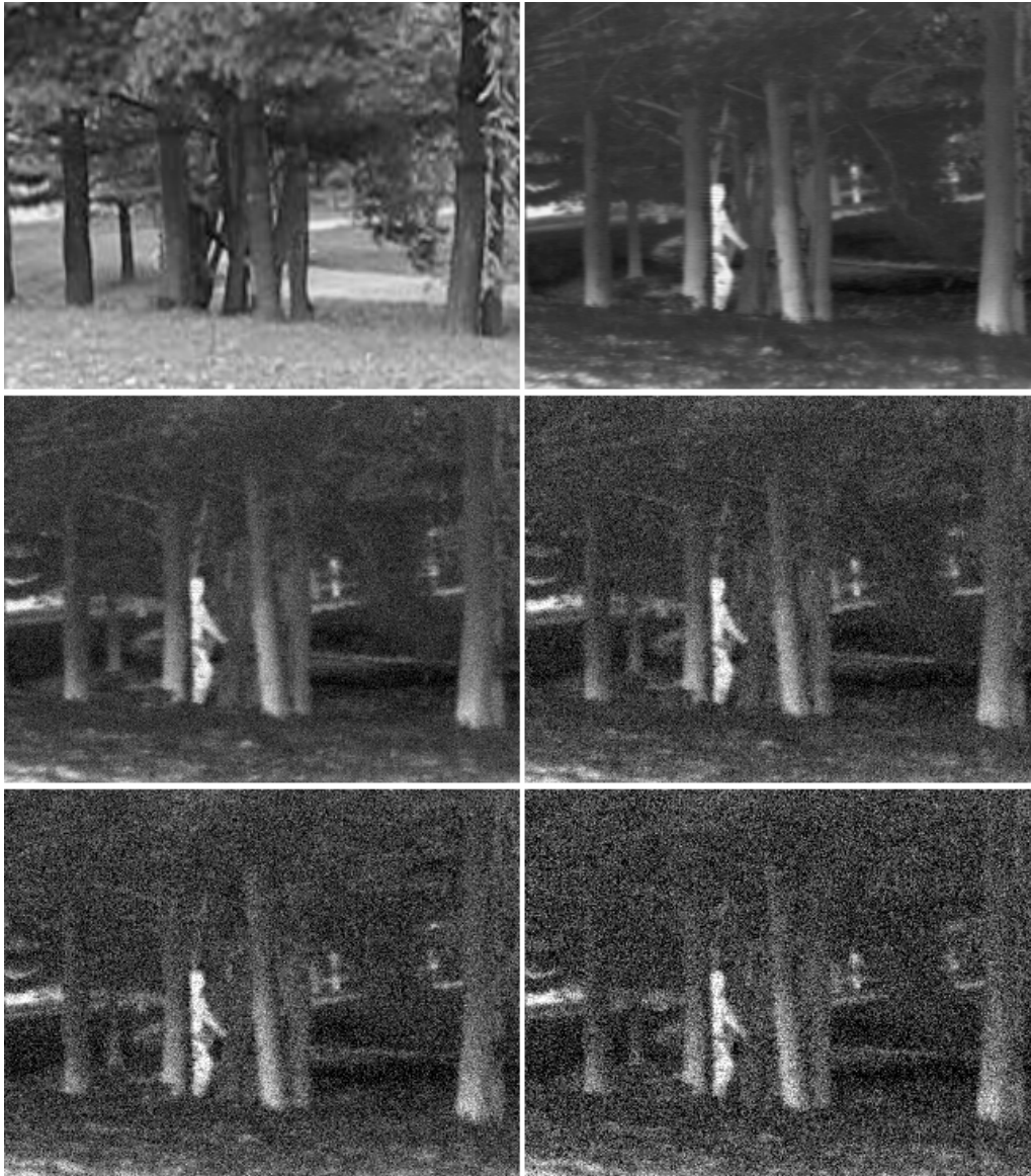
Figure 1. Corruption levels on “va1” sequence, visible reference top left, then from right to left noise free IR and at 10, 6, 3 and 1 dB SNR
