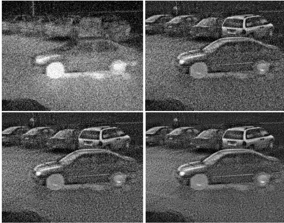
Figure 8. Input noisy thermal image at 1dB SNR and fused images using DT-CWT with select-abs-max feature selection followed (clockwise) by no, hard and soft thresholding
