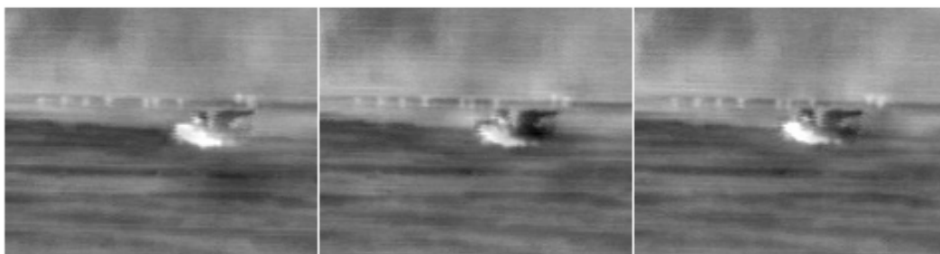
Figure 2. Consecutive frames from a fused sequence showing dynamic flickering induced by inconsistent feature selection
