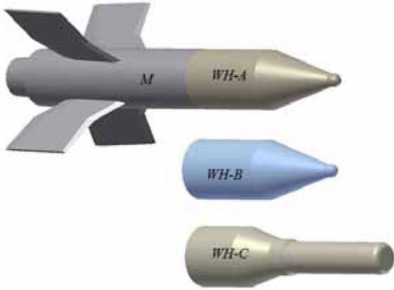
Figure 1: Modernization of the antitank missile with improved warheads
