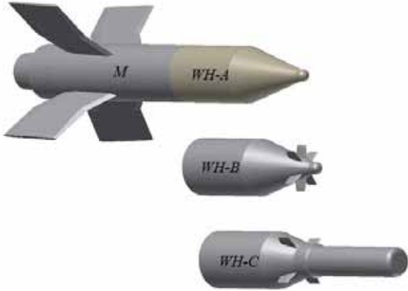
Figure 3. Aerodynamic configuration of the antitank missile with improved warheads
