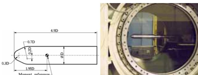
Figure 3. The blunted-cone-cylinder model
