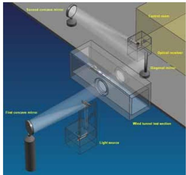
Figure 4. The Schlieren system of the T-38 wind tunnel
