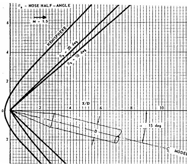
Figure 2. An example of a graph [3] showing the shape and position of the bow shock waves for hemispherical and two conical noses at Mach number 1.5 and 15 angle of attack (D=model diameter,  $\theta_s$ =nose half-angle,  $\alpha$ =model angle of attack, M=Mach number)
