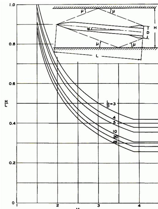
**Figure 1.** Maximum ratio of the model length and the span of the fins as a function of the free stream Mach number ( $L$ =model length,  $D$ =maximum model diameter,  $\mu$ =shock wave angle,  $H$ =test section height), [3]
