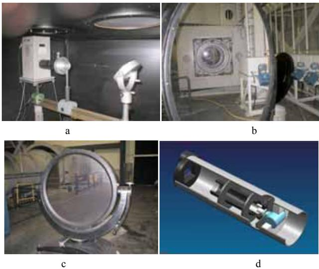
**Figure 5.** Parts of the T-38 Schlieren system: a – light source, b – diagonal mirror, c – second concave mirror (image forming mirror), d – optical receiver (shown as a CAD model in order to display it in a cross-section)
