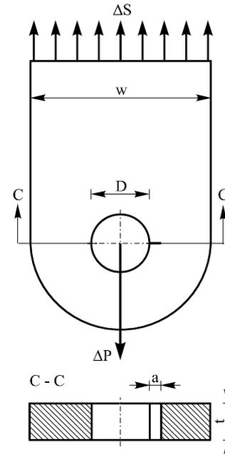
Figure 1. Geometry of a lug with through-the-thickness crack.
