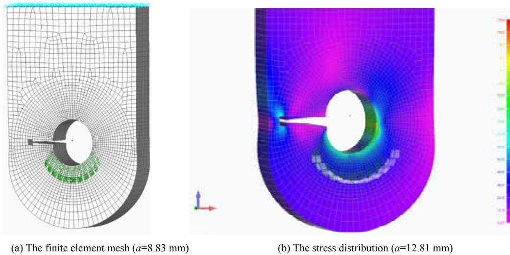
**Figure 4.** The lug with through-the-thickness crack subjected to cyclic axial loading.
