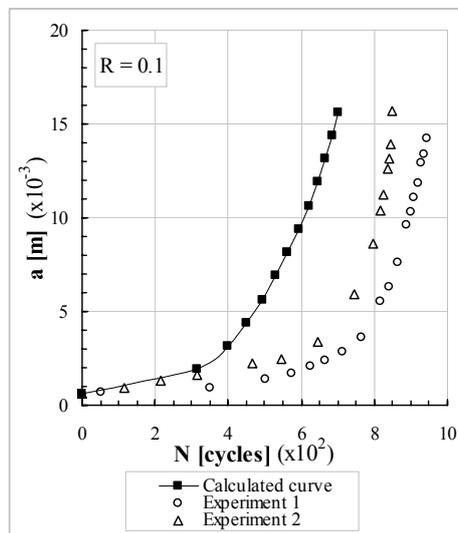
Figure 3. Crack length against number of loading cycles up to failure (1-ABPLC48, 2-ABPLC92. Experiments from Ref. [15]).
