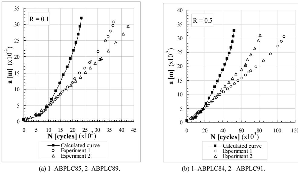
Figure 2. Crack length against number of loading cycles up to failure (Experiments from Ref. [15]).
