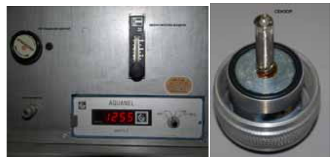
Figure 2. a) Front side of Aquanal hygrometer, b) Aquanal sensor
