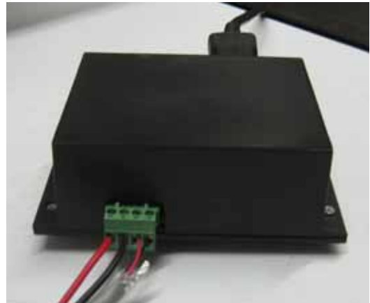
Figure 4. A voltage current converter mounted on the Aquanal hygrometer chassis
