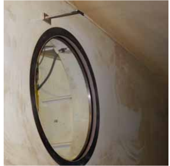
Figure 4. Pitot probes in the settling chamber (left) and in the test section (right) of the T-38 wind tunnel.
