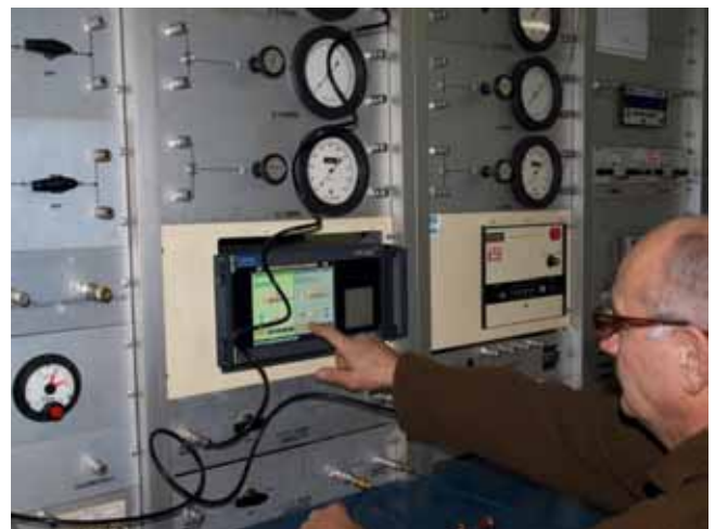
Figure 10. Preparation for calibration with the CPC6000 in the pressure laboratory
