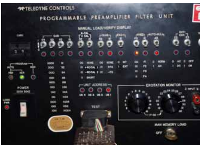
Figure 11. Front panel of the analogue unit of the Teledyne data acquisition system
