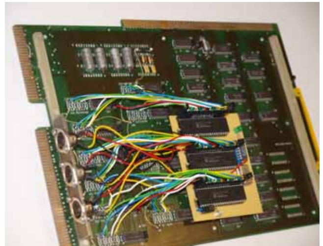
Figure 12. Prototype of the RS-485-to-parallel interface piggy-backed on a parallel-digital-input card of the Teledyne data acquisition system
