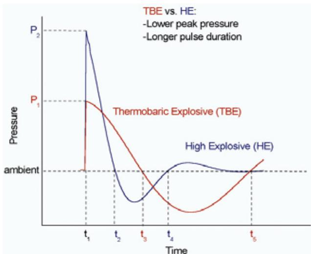
**Figure 1.** Pressure – time dependence of high explosive (HE) and thermobaric explosive (TBE) detonations
