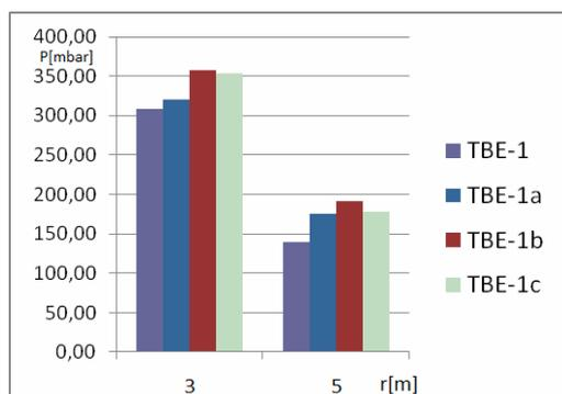
Figure 11. Pressure impulse at 3m and 5m for TBE-1, -1a, -1b, and TBE-1c
