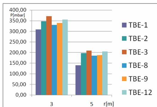
Figure 10. Pressure impulse at 3 m and 5 m for TBE-1, -2, -3, -8, -9 and TBE-12
