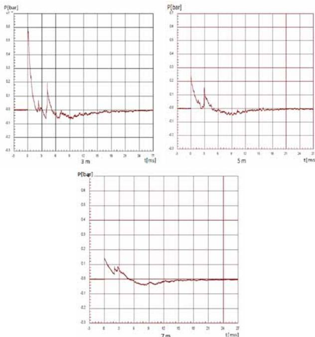
**Figure 5.** Dependence  $\Delta p = f(t)$  for TBE-2 at distances 3, 5 and 7 m, respectively
