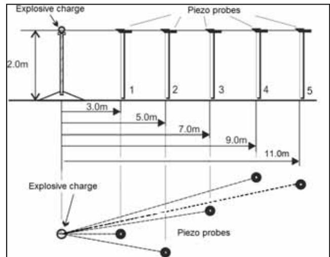
Figure 4. Scheme of the experimental determination of the ASWF parameters
