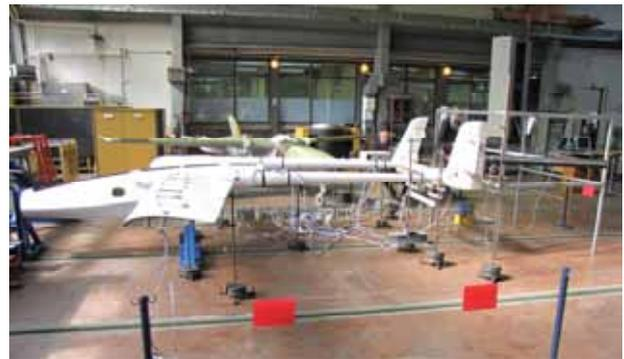
Figure 7. Static strength testing of UAVs
