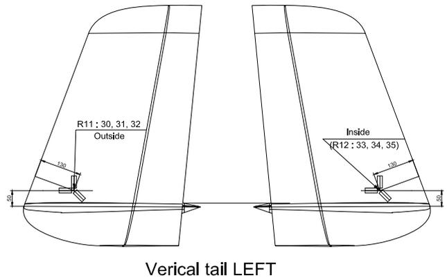
Figure 12. Disposition of the stain gages on the left vertical tail
