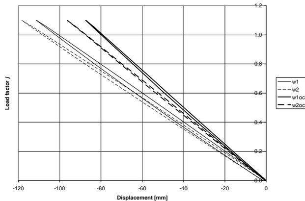
Figure 16. Vertical displacements on measuring positions 1 and 2 (cleaned)
