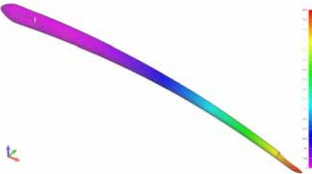
Figure 3. Tail beam displacements ( $w_{max}=84.83$  mm),  $j=1.0$
