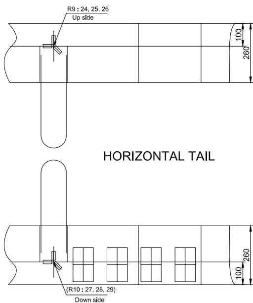
Figure 10. Disposition of the stain gages on the horizontal tail
