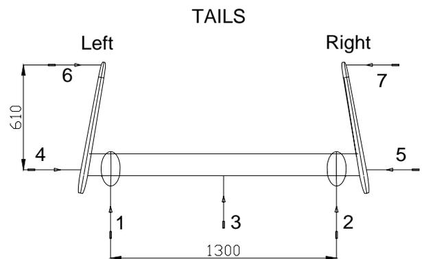
Figure 14. Sensor displacements on the horizontal and vertical tails
