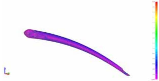
Figure 6. Tail beam stresses  $j=1.1$  (55daN), Von Mises=26.69 hbar
