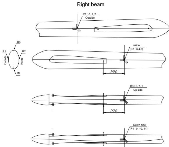
Figure 8. Disposition of the stain gages on the right beam
