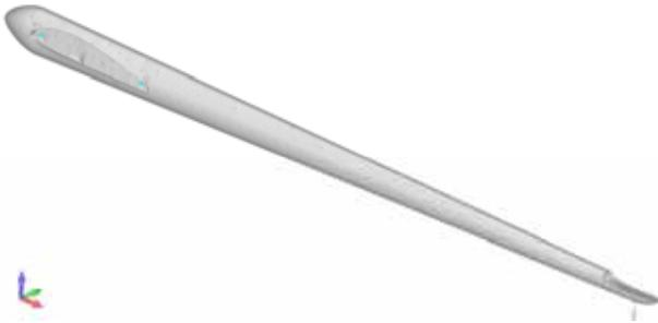
Figure 2. Finite Element Model of the UAV tail beam
