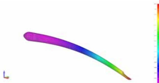
Figure 5. Tail beam displacements ( $w_{max}=93.32$  mm),  $j=1.1$  (55daN)
