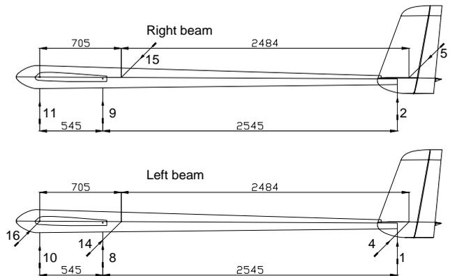
Figure 13. Sensor displacements on the beams
