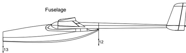
Figure 15 .Sensor displacements on the fuselage
