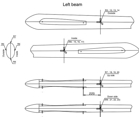
Figure 9. Disposition of the stain gages on the left beam
