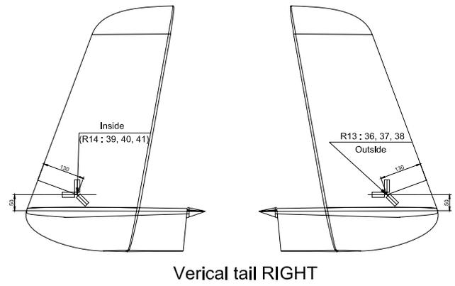
Figure 11. Disposition of the stain gages on the right vertical tail
