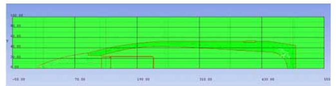
Figure 7. Initial 2D model of the 105 mm HE projectile generated in the coupled Euler-Lagrange mesh (axial half-section)
