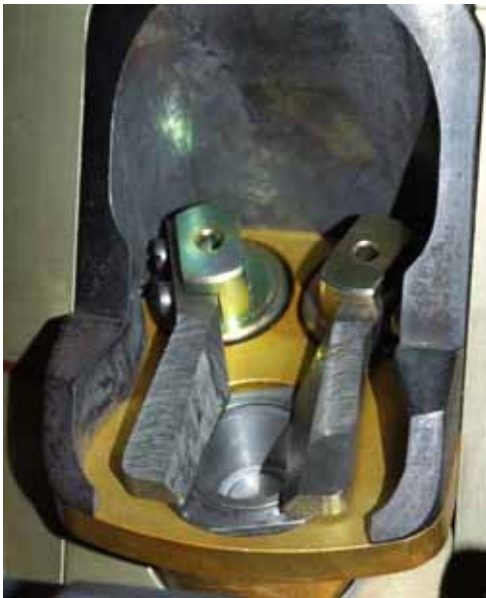
Figure 16. Bumar nozzle exit with the jet tabs
