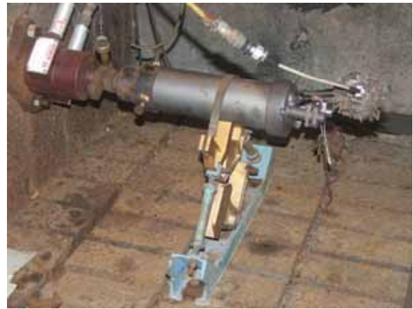
Figure 20. Experimental Maljutka sustainer rocket motor on the one-component test stand
