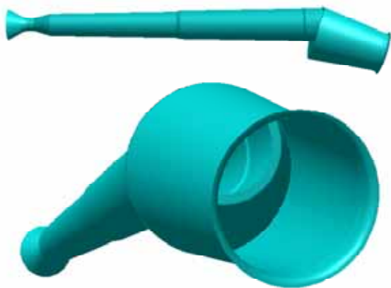
Figure 25. Maljutka (the sustainer rocket motor) – The flow space geometry: nozzle and deflector
