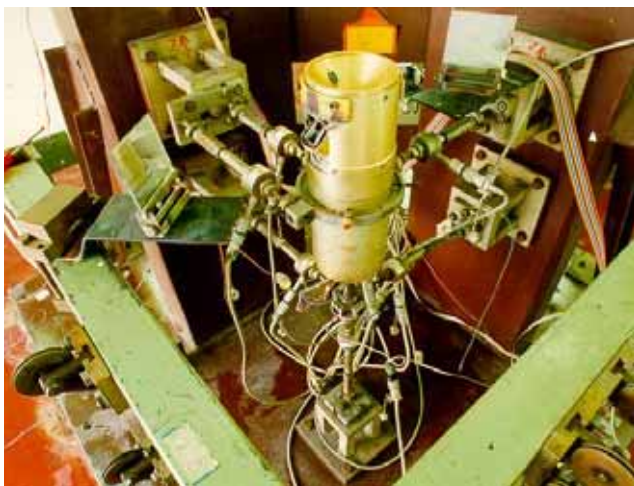
Figure 2. Bumbar sustainer motor on the 6-K test stand
