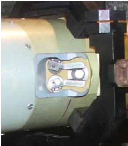
Figure 8. Bumbar, the nozzle with the interceptors
