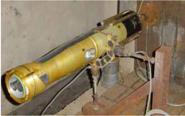
Figure 6. Bumbar test rocket on the 3-K test stand
