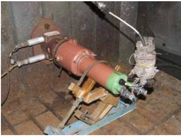
Figure 28. Maljutka sustainer rocket motor on the one-component test stand
