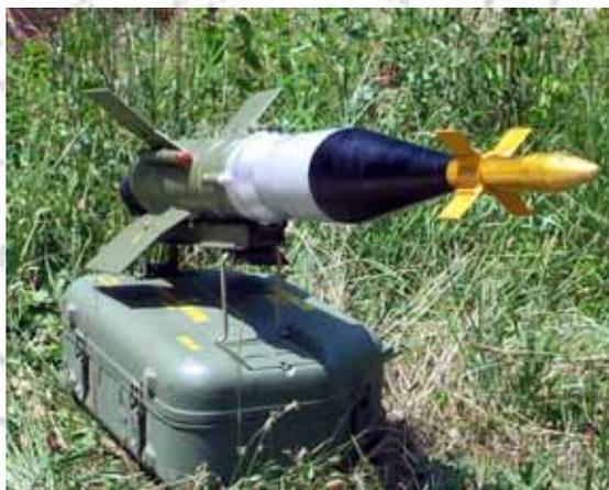
Figure 25. Antitank launching kit MALJUTKA-2T with the tandem warhead
