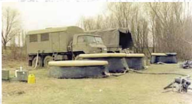
Figure 68. Water station for complex water purification
