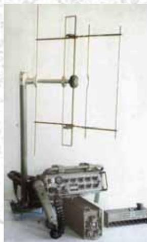
**Figure 55.** Radio-relay device RRU-1
