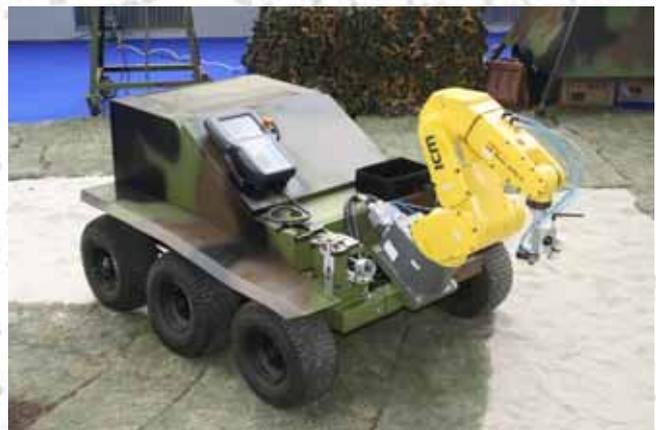
Figure 67. TORO robotised demining vehicle
