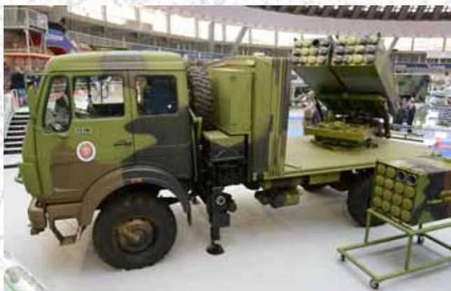
Figure 23. Modular multi-launch self-propelled rocket system LRSVM (MORAVA)
