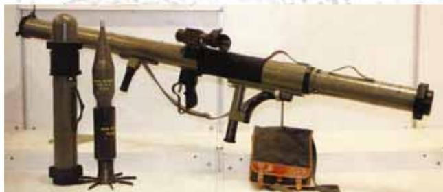
Figure 24. 90 mm portable rocket launcher M79 OSA
