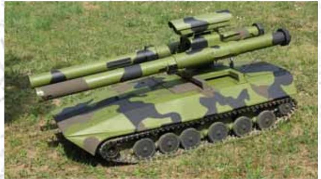
**Figure 28.** Mobile modular robotized anti armour system MILICA
