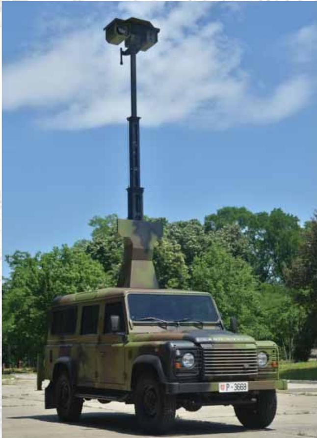
Figure 60. MIP-11 multi-sensor intelligent platform
