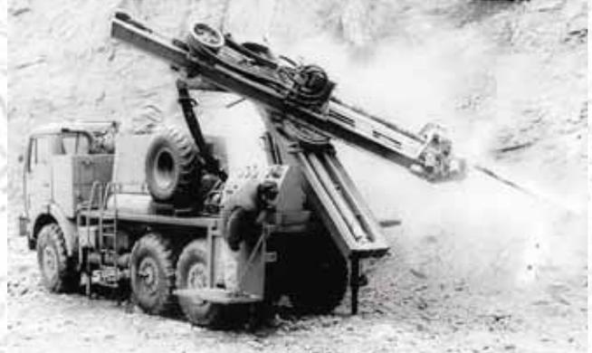
Figure 66. M70 drilling kit for mine wells
