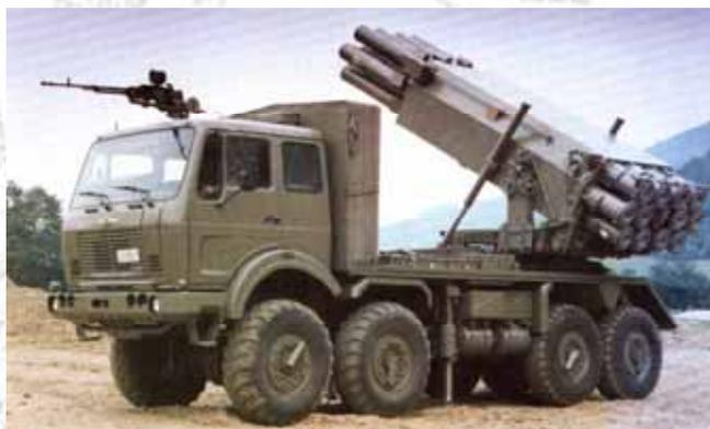
Figure 21. Self-propelled multilaunch rocket system M87 ORKAN
