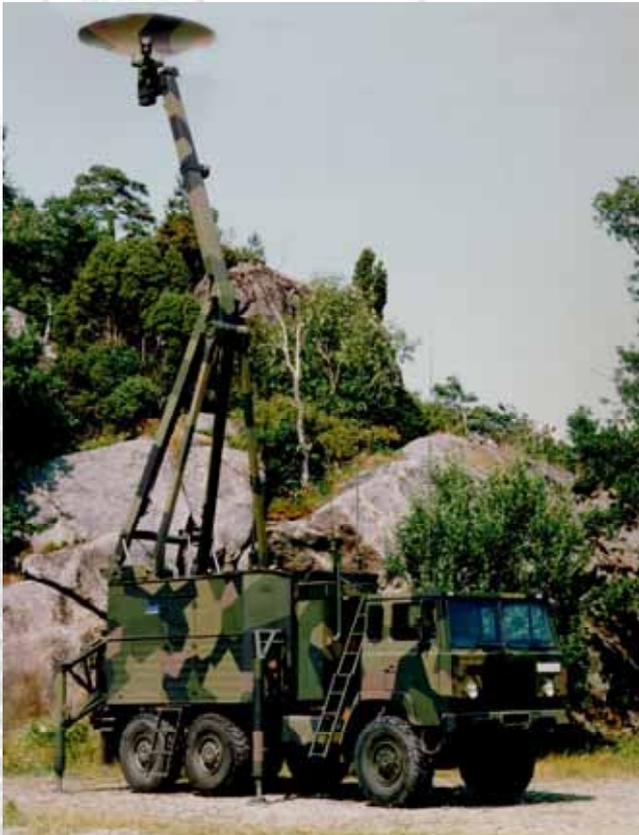
Figure 57. GIRAFFE radar system
