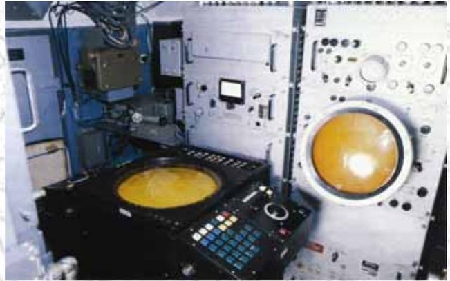
Figure 58. Control board of the surveillance-acquisition radar P-15 in the SONIC system
