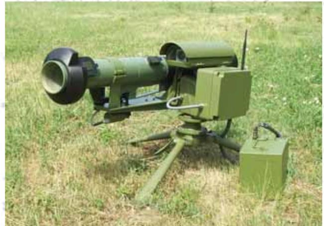
**Figure 29.** Stationary modular robotized ant armour system APOS
