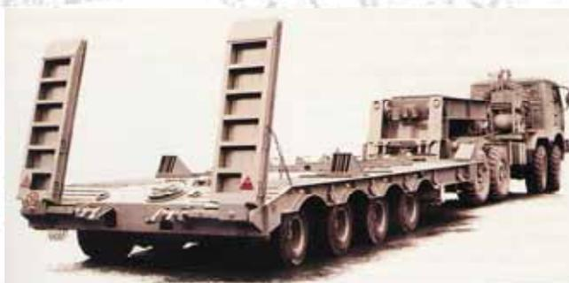
**Figure 39.** Towed vehicle FAP 3232 with a low-carrying semi-trailer with a capacity of 45 t
