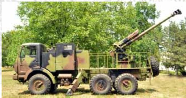
Figure 10. 122mm self-propelled howitzer SORA
