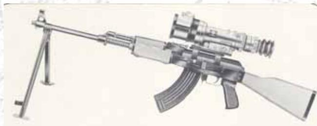
Figure 3. Machinegun M72 with passive night sight
